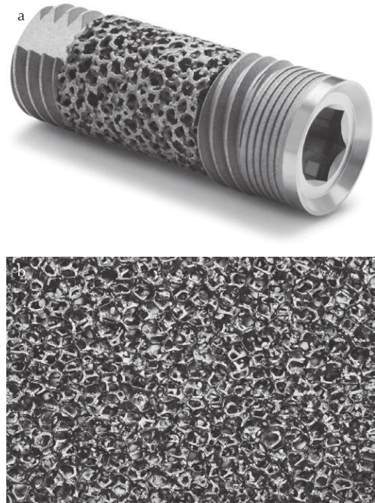
2.13. (a) Zimmer ® trabecular metal ™ surface. (b) Micrograph of trabecular metal ™ surface texture (courtesy of Zimmer Dental)
